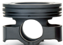
Monotherm® diesel engine piston from Mahle: reducing friction loss and weight while improving thermodynamics yields total fuel savings of approximately 3 % in the NEDC*. *NEDC (New European Driving Cycle)
