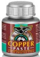
COPPER PASTE forms an effective separating layer between metal surfaces, thus preventing corrosion, at temperatures from -40°C to +900°C, and up to +1200 °C for short periods. The paraffinic base oil works at temperatures up to 280°C. Above this, lubrication is guaranteed by the copper particles. At the same time, these particles provide effectively treated parts with optimum corrosion protection. Assembly paste for all kinds of screws, threads and press fits.
