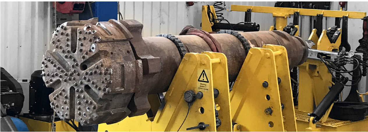
At the press of a button, even badly seized drill heads can be released.
