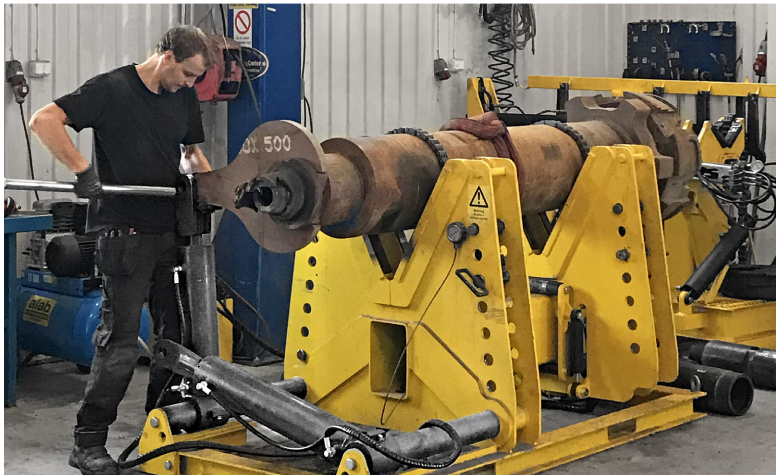
The hydraulic fluid transmits forces of up to 30 tonnes in the thread-loosening process.
