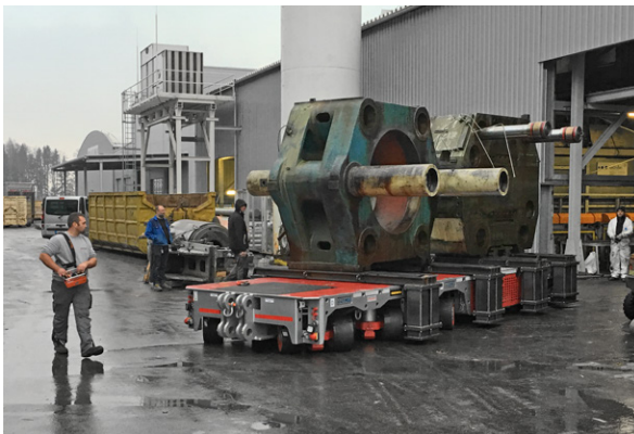
The self-propelled industrial dolly can move loads up to 175 tonnes and is steered by remote control.
