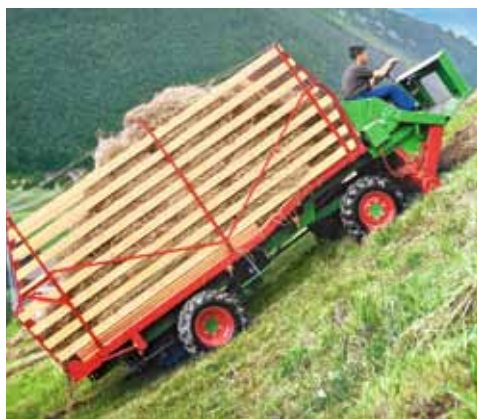
The Schilter LT 2 forage wagon picks up clippings before they reach the front axle. This is a huge benefit in terms of feed cleanliness.
