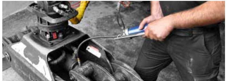
The operator's duty: regular lubrication. Here GREASE 190 is being applied to the joint of a loading crane grab.
