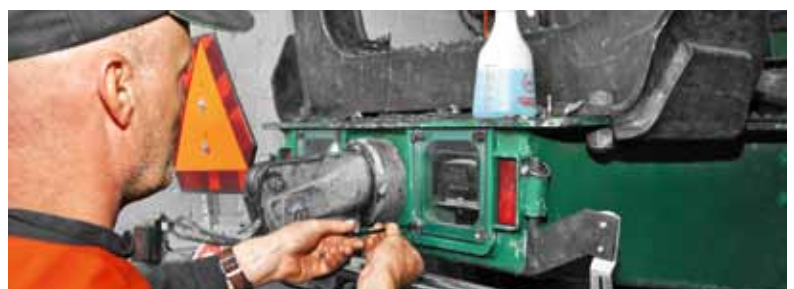
Cleaning the backup camera: a little windshield washer fluid and a few minutes' work are enough to ensure a clear rear view.
