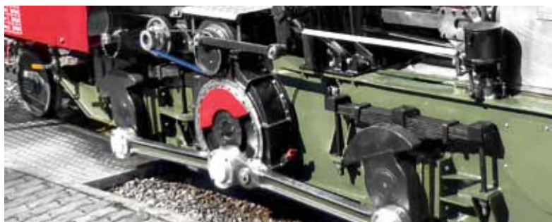
Good to see: the supply tank, mounted right next to the grease lubrication pump (in photo at right on top).
