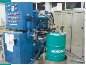
**MOTOREX OEKOSYNT HEES successfully** passed the rigorous 1,300-hour endurance test at Bosch Rexroth.
