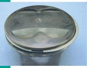
The piston also still looked quite good after the test, with wear parameters within the applicable tolerances.
